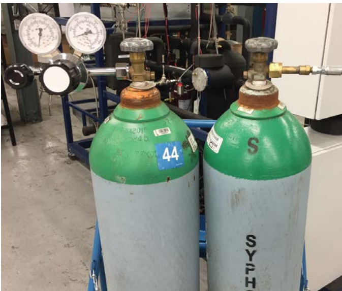
Figure 25. Example of R-744 charging equipment
